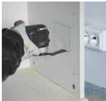
Plunge cutting in wood or metal, e.g. for removing window frames or door frames
