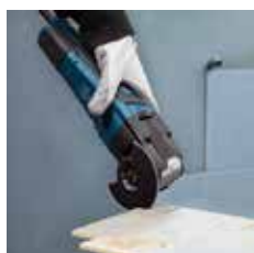
Making smaller cutouts precisely in soft wall tiles
