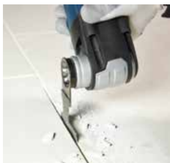
Removing stubborn mortar or tile adhesive, e.g. when replacing damaged tiles
